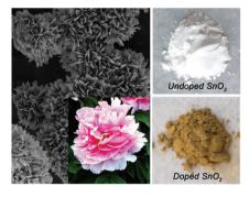
Flower-like hierarchical  $SnO_2$  nanostructures are assembled from single-crystal-line  $SnO_2$  nanosheets with high-index (11 $\bar{3}$ ) and (10 $\bar{2}$ ) exposed facets.  $Sn^{2+}$  self-doping leads to formation of tunable oxygen vacancy bandgap states and extended absorption in the visible spectral range. This work highlights the possibility of simultaneous engineering of surface energetics and electronic properties of  $SnO_2$  based materials.
